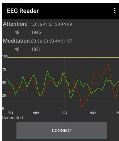
Fig. 5, This was the image of the reader when the task was finished. We can see the concentration went to the lowest trough when the task was concluded and went to almost the maximum when the subject had stopped completely.
